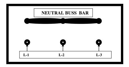
L-1 TO L-2 = 208 VOLTS L-2-TO L-3 = 208 VOLTS L-3 TO L-1 = 208 VOLTS
