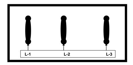
L-1 TO L-2 = 120 VOLTS L-2 TO L-3 = 120 VOLTS L-3 TO L-1 = 120 VOLTS
